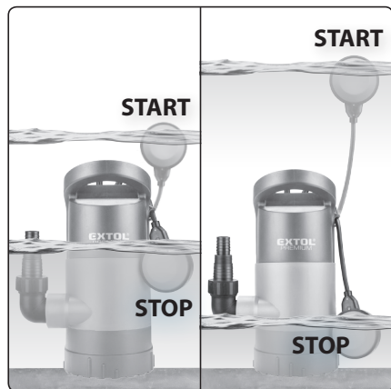
Fig. 4, Illustration of float switch function
